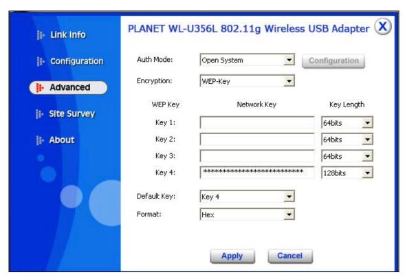
Additional security can be achieved by using any of the following encryption methods: WEP (Wired Equivalent Privacy), WPA and WPA2 (Wi-Fi Protected Access), and WPA-PSK and WPA2-PSK (Pre Shared Key).
